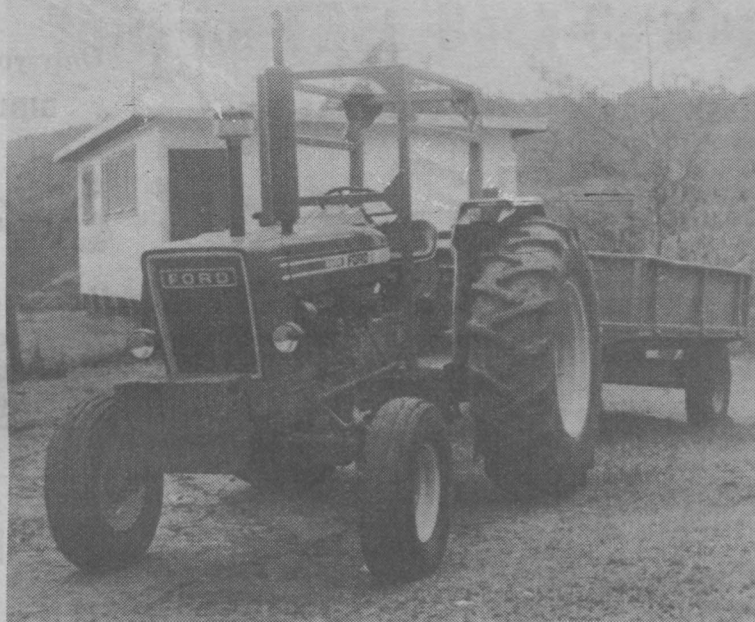
This is a view looking at the front of the new tractor and also showing the Hornibrook 3 1/2-ton heavy-duty dump type trailer hooked to the tractor.
